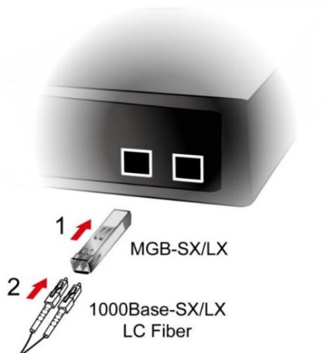
Figure 2-16 Plug in the SFP transceiver
